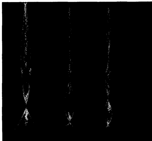
Fig. 1. Time exposure photographs show stable resonances of a rotating flexible chain.
