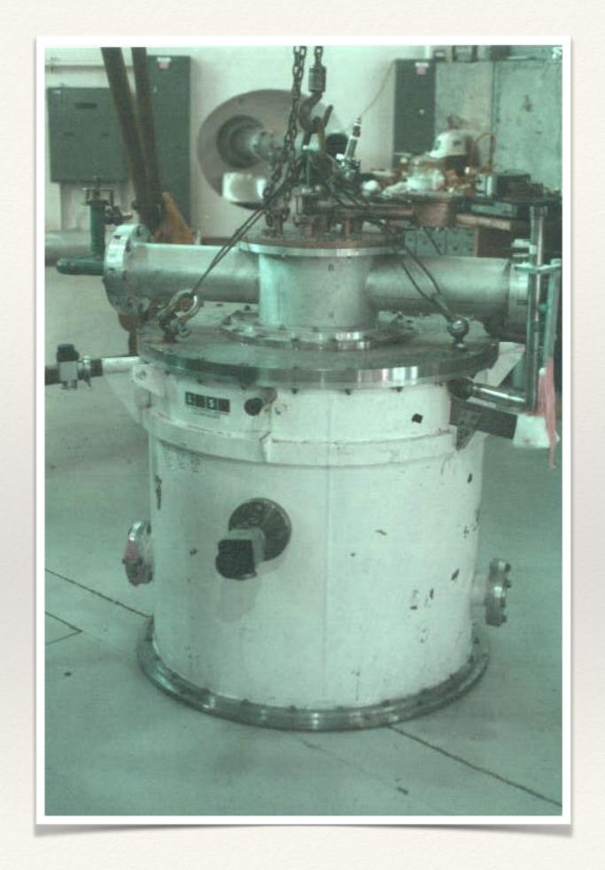
Polarized Target Cryostat
