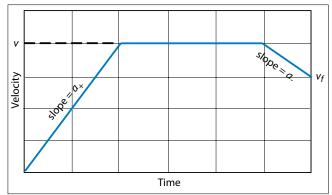
Fig. 1. The velocity-time graph for the kinematic model. It is the shape of the curve that describes the kinematic model, so units are omitted.
