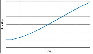
Fig. 2. The resulting position-time graph from the velocity-time graph of the kinematic model. Units are again omitted. Note the time axis is shifted from Fig. 1 due to the lead-off distance.
