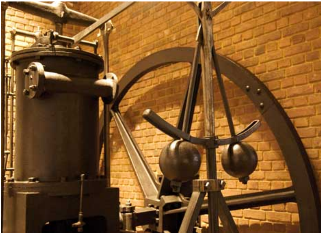
FIG. 2: Machines using the flyball governor
