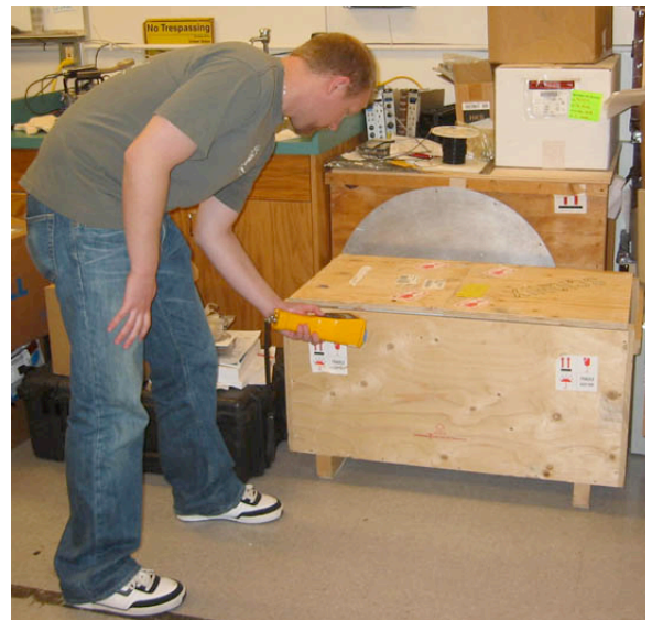
A packing case for the presence of nuclear material using a commercial, hand-held, low-resolution gamma-ray detector, commonly employed by first responders.
