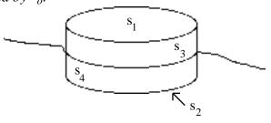
we choose a gaussian surface that straddles the surface of the conductor. We choose it in such a way that surface 1 is parallel to the local surface of the conductor. The total flux leaving the surface is just the sum of the fluxes leaving the four surfaces shown.
