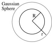
$\circ \vec{E} \cdot d\vec{A} = \circ E dA$  because E and dA are parallel.
