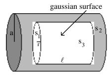
The integrals over  $s_1$  and  $s_2$  are both zero because the field is radial which means that no flux exits these faces (E is perpendicular to dA). Over  $s_3$  E is constant and parallel to dA so that integral is,  $\vec{E} \cdot d\vec{A} = E A = E2 \ r\ell$ .
