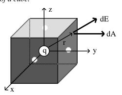
The flux through any closed surface is proportional to the charge contained inside.
