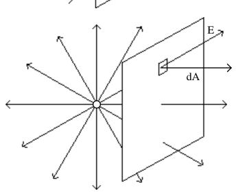
Example 1: Find the flux that exits a sphere centered at the origin due to a point charge also at the origin. A small surface area on a sphere is,  $d\vec{A} = r^2 \sin d d \hat{r}$ . Using the field due to the point charge,  $\vec{E} = k \frac{q}{r^2} \hat{r}$ , the flux can be calculated from its definition,  $\vec{E} \cdot d\vec{A}$ ,  $k \frac{q}{r^2} \hat{r} \cdot r^2 \sin d d \hat{r}$  $= k q \sin d \int_{0}^{2} d = 4 kq = \frac{q}{r^2}$
