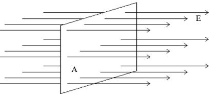
If a constant field is at an angle from the normal to the surface, then the flux is given by  $= EA \cos = \vec{E} \cdot \vec{A}$ .
