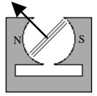
A galvanometer measures current by allowing the current to flow through a coil of wire creating a magnetic dipole. The coil is placed in a magnetic field of the proper shape so that the torque doesn't depend on the angle the loop makes with the horizontal. The torque on a dipole is,  $\vec{=} \vec{\mu} \times \vec{B} = \mu B$ . In terms of the magnetic moment of a loop of N coils, = NIAB. Notice that this is linear in the current (Twice the current produces twice the torque).
