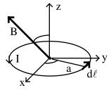
What about the torque on the loop? The book wimps out and does a square loop. We're tough, so let's do a circular loop of radius, a. The loop will be in the x-y plane and B is in the x-z plane and angle from the z-axis. This geometry means no loss of generality.
