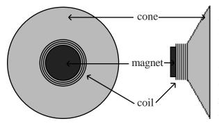
A magnet is mounted to the frame of the speaker and a coil of wire is mounted to the cone. The current from the amplifier is sent through the coil. When the current is one direction the force on the coil is one direction. When the current reverses, the force on the coil reverses. The resulting oscillatory motion of the cone creates the sound waves.
