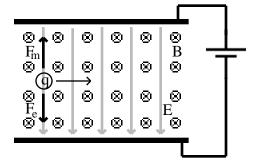
Example 4: A mass spectrometer requires charged particles traveling at  $2.00 \times 10^5 \text{ m/s}$ . The magnetic field in the device is 0.500T. Find the potential difference across the plates of the velocity selector given their separation is 0.800cm. Applying the Second Law,  $\vec{F} = m\vec{a}$  q B – qE = 0 =  $\frac{E}{B}$ . Between parallel plates, E =  $\frac{V}{d}$ . Finally, =  $\frac{E}{B} = \frac{V}{Bd}$  V = B d = (0.500)(2.00 \times 10^5)(8.00 \times 10^{-3}) = <u>800V</u>
