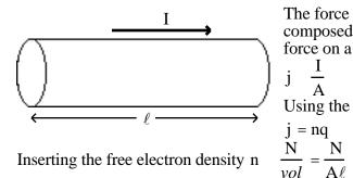
The force on a current carrying wire is  $\vec{F} = \vec{I\ell} \times \vec{B}$ . The current is composed of individual charges. We want to know the magnetic force on a single charge. Recall the definition of current density,
