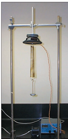
Fig. 2. The mass-spring system with PASCO function generator and motion detector.
