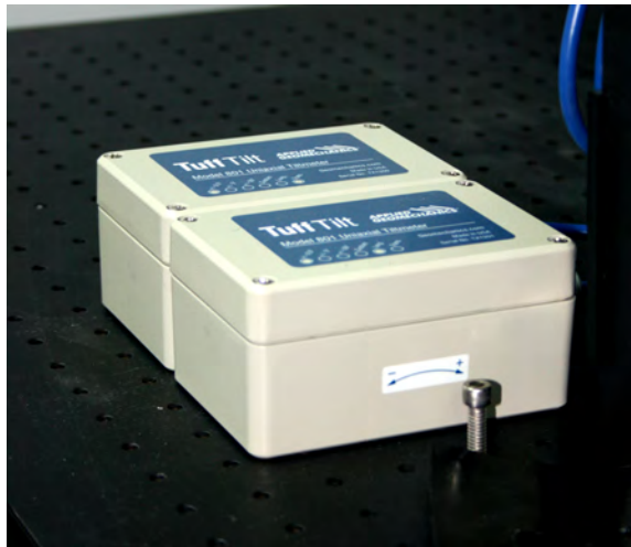
Fig. 8. Photograph of the two gravity referenced tiltmeters. The sensors measure pitch and roll angles of the instrument to 10^{-6} of a degree.
