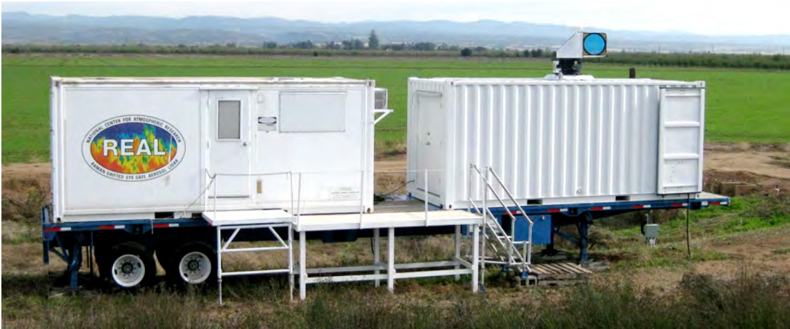
Fig. 4. Photograph of lidar at the CSUC farm. The container on the left is used as a field office. The container on the right houses the lidar. The BSU is on the top of the right container.
