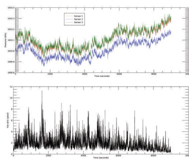
A long data run in environmental conditions (AKA "outside on the dirt") reveals a wealth of data and definite correlations between wind events and pressure-fluctuation changes.
