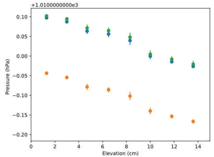
To verify that these sensors were able to do what was needed, we recorded pressure measurements as we increased the height of the instrument. (Yes, the total elevation change in this graph is just 15 cm!)
