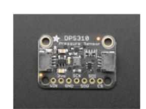
The sensor that we are using is an Infineon DPS310. For this test board we purchased them pre-installed on a breakout board from Adafruit. The manufacturer claims 0.002hPa precision and  $\pm 1hPa$  absolute accuracy.
